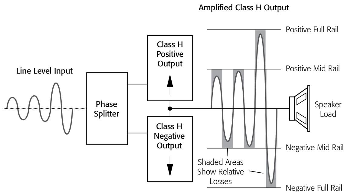
Figure 2 - Class H Amplifier with Losses
