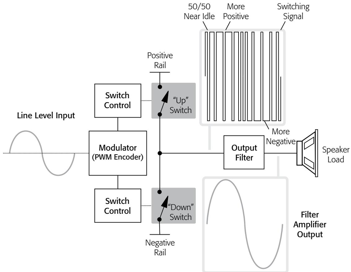
Figure 3 - Class D Amplifier with Modulation
