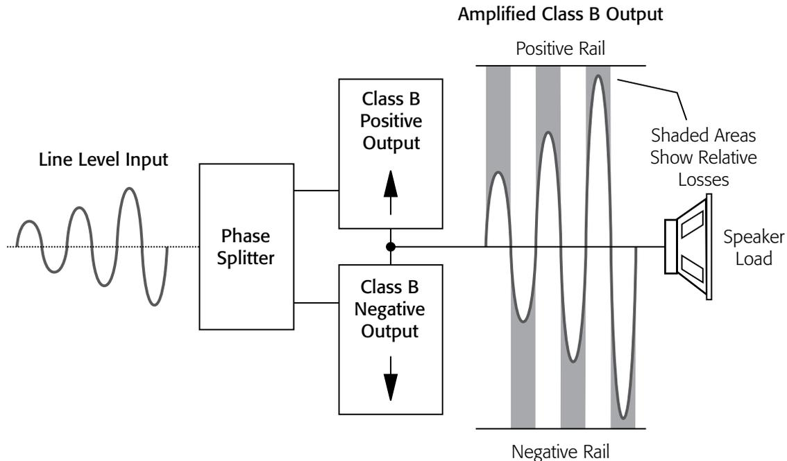
Figure 1 - Class B Amplifier with Losses
