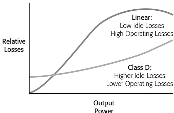
Figure 5 - Linear vs. Switchmode Loss Curves
