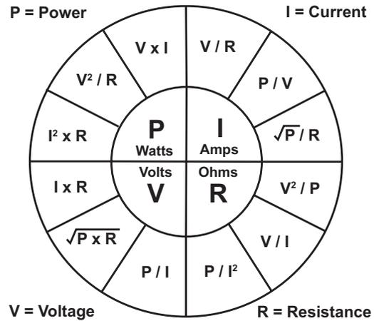
The amount of power that is delivered to a load is governed by two laws – Ohm's law and Joule's law. Ohm's law states that in order to drive a specific current through a specific resistance or load requires a specific voltage.
