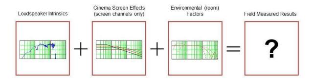
**1. Loudspeaker Intrinsics** – These refer to inherent characteristics of the loudspeaker and its components. These intrinsics are the result of natural physics; with current transducer technology, they are unavoidable, regardless of quality or cost. These intrinsics result in frequency response anomalies which cannot be corrected in the field, since their effects cannot be isolated from the other causal factors in the room.
