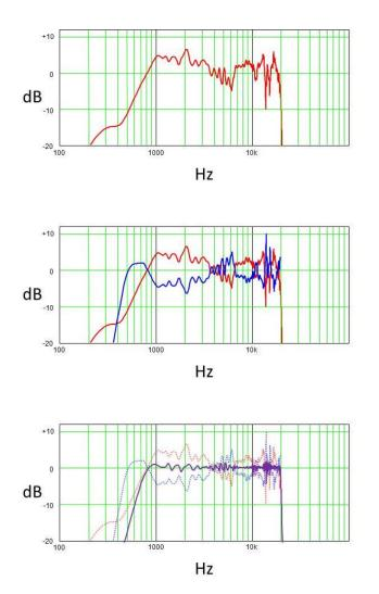
A curve is generated representing the unaltered response of the loudspeaker (top, red line). Then, an inverse of that response is created using FIR filters (middle, blue line). When the two are combined, the result is a much flatter response (purple line, bottom).
