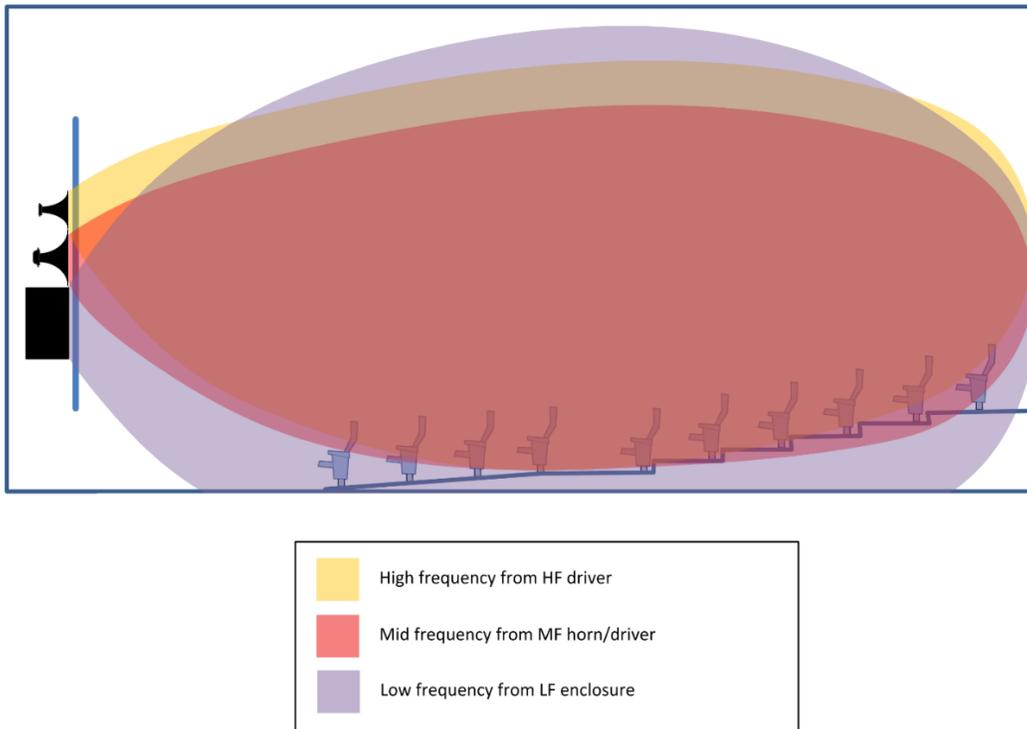
Fig. 2. Conventional multi-way screen channel loudspeakers project low, mid, and high frequencies evenly from a single source location.
