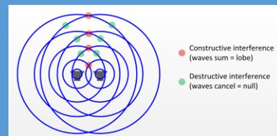
Multiple lobes and nulls are created at different physical locations relative to the sound sources, and are both frequency and level dependent.
