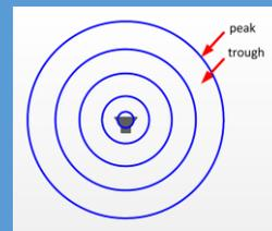
When the compressions meet at the peak of the wave cycle, constructive interference occurs, and a lobe is formed producing higher sound pressure level in that region. Likewise, when two troughs meet, it also creates constructive interference. When a peak from one sound source meets the trough of a wave cycle from another sound source, destructive interference occurs, and a null is formed.
