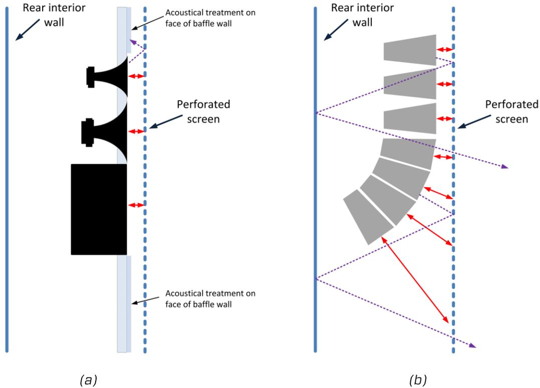
Fig. 5. A multi-way screen channel loudspeaker mounted in a full baffle wall (a) with acoustic absorption minimizes behind screen reflection and potentially destructive interference and comb filtering. A curved line array (b), with no baffle wall and increasing distances from the rear of the screen, creates multiple reflections of different path lengths and time arrivals.
