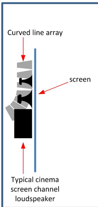
*Fig. 3. A curved line array requires more space behind the screen compared to a typical multi-way screen channel loudspeaker.*
