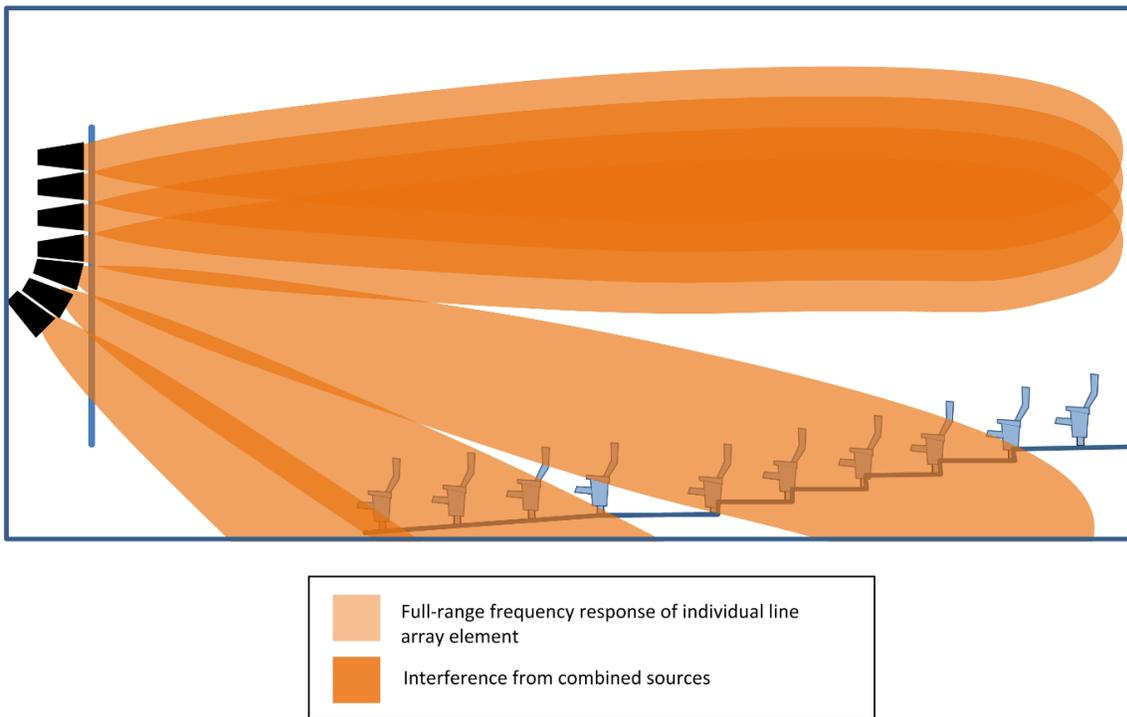
Fig. 7. A line array system projects the same signal source from multiple elements, which can result in nulls and significant pattern overlap and combing, due to interference at various wavelengths.
