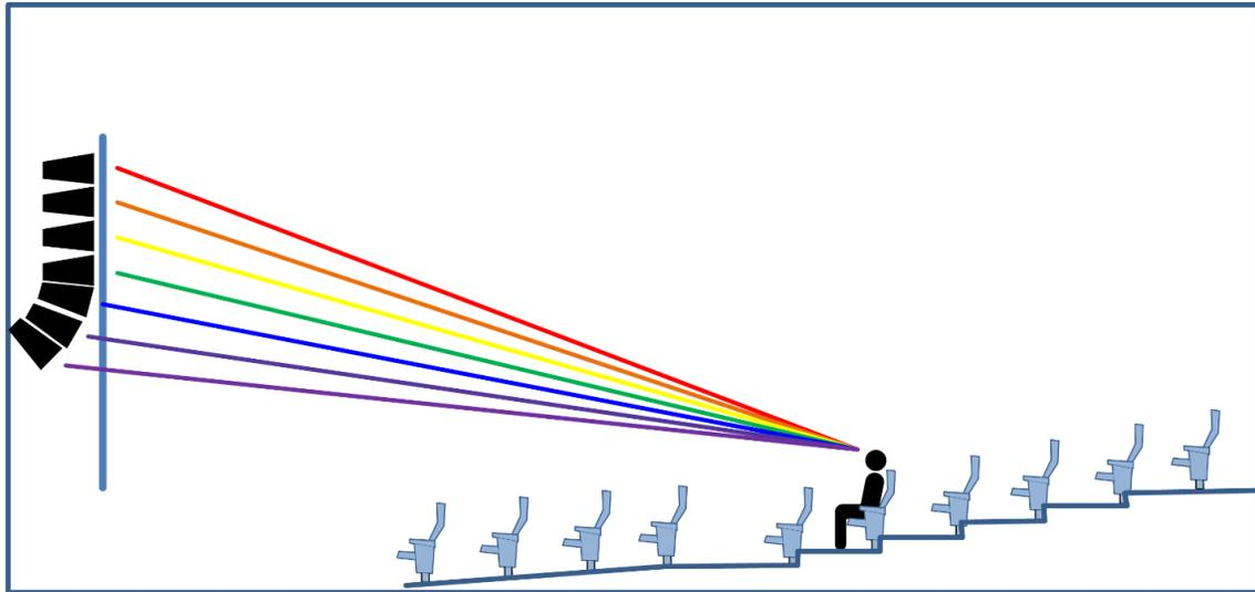
Fig. 6. The distance to a listener from each line array element is different, which can result in “blurred sound”, or smearing.
