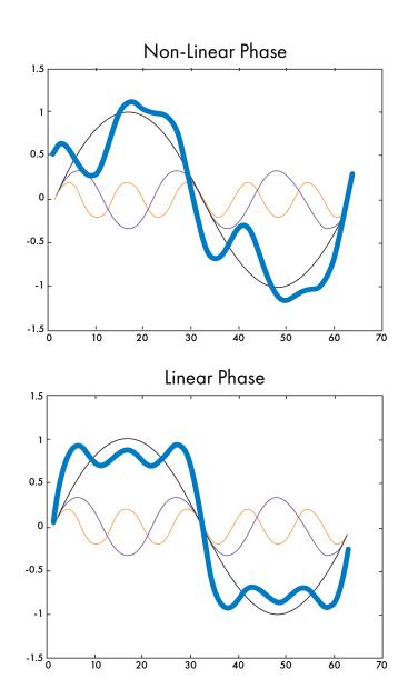
In a system with non-linear phase, the time relationship between fundamental and harmonics is altered and something other than a square wave emerges at the output. Another term for altered waveform is distortion.
