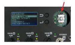
2. Use a flat tool to carefully pry the knob off the rotary encoder on the loudspeaker's amplifier module. You will see a micro USB port next to the rotary encoder. Plug the cable into the port and plug the other end into an available USB port on the computer.
