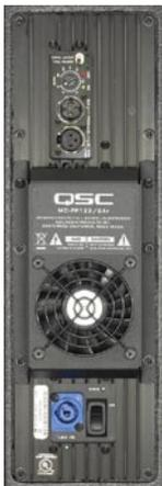
QSC's PM series are the most compact, lightweight and efficient loudspeaker power modules currently available. They have been specifically developed to meet the headroom and voltage swing requirements of high-end professional loudspeaker systems. The PM1000 features two channels producing 800 watts (LF) and 200 watts (HF) respectively, while the PM1400 delivers 1400 watts into a single channel.
