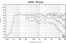
Frequency Response, passive mode (O°, 40°, 80°, 120° horizontal axis)
