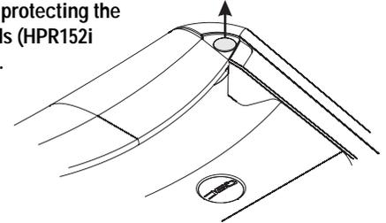
Rubber insert removal (HPR152i and HPR153i only); gently pry upward to loosen insert.
