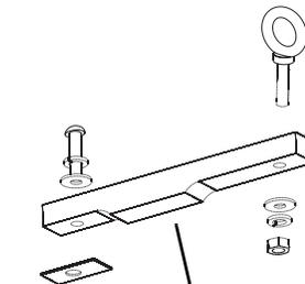
Installation of pull-back bar above the enclosure.
