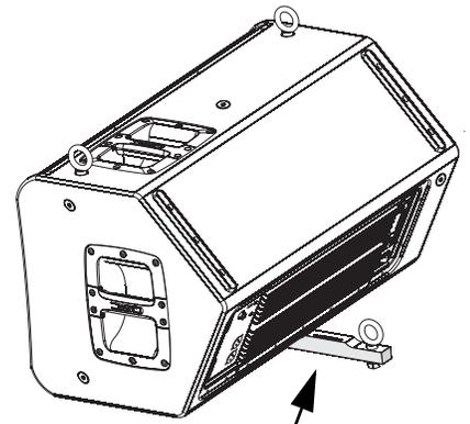
Pull-back bar assembly- Note location of offset cut-out on bar and orient to enclosure shape according to which side it is mounted on. Adhesive gasket is to be used between the bar and the enclosure. Ensure use of flat and lock washers in order shown. Tighten all hardware.
