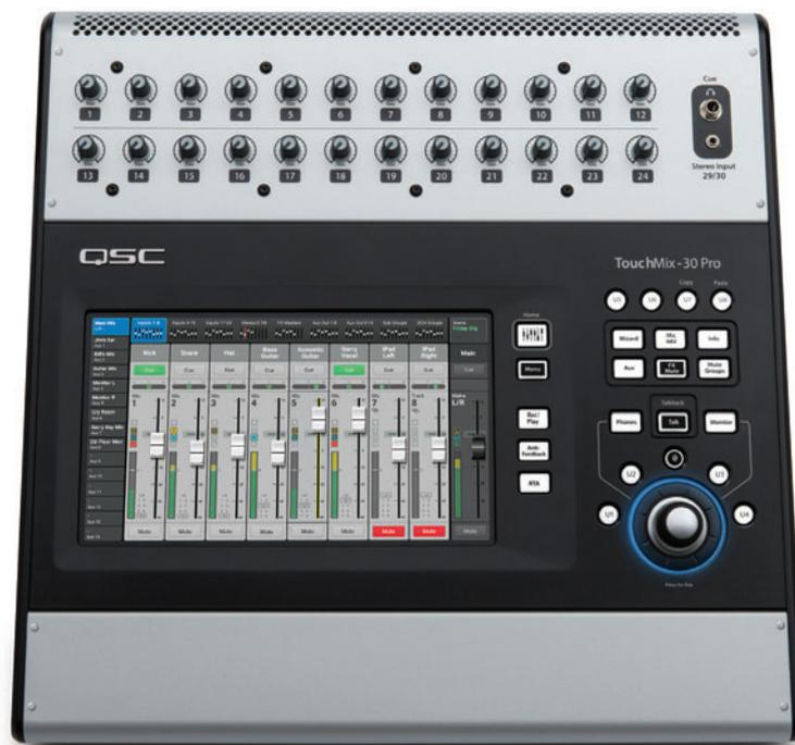
Once you've roughed in your mix, the TouchMix-30 Pro has six independent FX engines plus Pitch Correct, which could be used to fix intonation or detune instruments or vocals for a thickening effect. You don't need to give up any aux mixes to use all of the FX, and the presets can also be altered and saved to the console's preset folder or any drive connected via the USB port.
