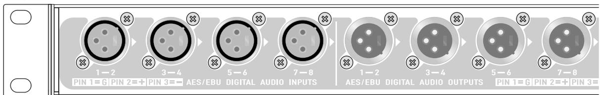
Channel numbers and connector pinouts are labeled on the rear of the unit, as shown in the illustration above.
