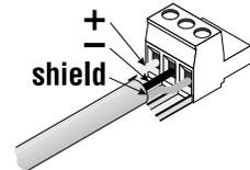
**To connect unbalanced inputs:** insert the signal conductor into the + terminal and the shield to the - terminal, with a jumper to the ground/shield terminal, as shown at the lower right.
