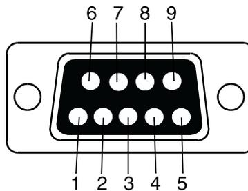
Pins 1 (DCD), 4 (DSR), and 6 (DTR) are tied together. Pins 7 (RTS) and 8 (CTS) are also tied together. DCE (receives on TD) operation; parity bit not checked.
