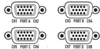
To connect the cable, orient the connector properly, then push into the receptacle until it is firmly seated; tighten the retaining screws "finger tight".
