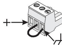
**Omni In connections.** Variable input must be 10k ohm variable resistor. Contact closure input can be a switch or relay contacts. These inputs can operate software "devices". Negative (-) terminal is at chassis potential.
