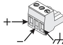
**Analog audio input-unbalanced connection.** Note jumper wire between - and ground.
