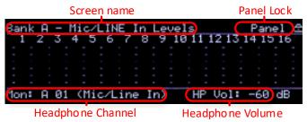
There are two views for bank metering. The main part of each bank view shows meters for each analog input or output in that bank. This view can be used to select the monitor output if the panel lock is not active by pressing in the "Menu Nav" button. This activates a cursor that can be scrolled used the knob to select one of the visible channels. Once the desired channel is selected, press the separate "Monitor Select" button and that channel will when be routed to the headphone output.
