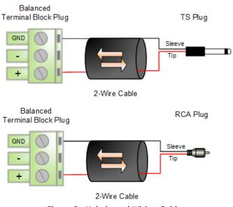
Figure 3 - Unbalanced Wiring Guide
