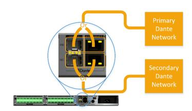
Figure 4 -"Redundant" mode, no daisy chain
