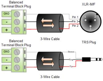
Figure 2 - Balanced Wiring Guide
