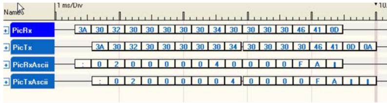
the PIC at all. . Note that this record sets an extended linear address and does not actually program
