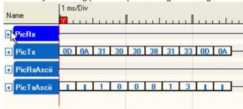
Characters except CR are immediately echoed. CR is echoed after the line of text has been interpreted. A LF is transmitted after the echoed CR.
