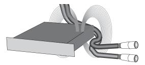
Magnetic field from power supplies in equipment can induce hum into cabling that is located in the field. If hum is a problem, try relocating cabling so that is away from power supplies, transformers and other magnetic field producing devices.
