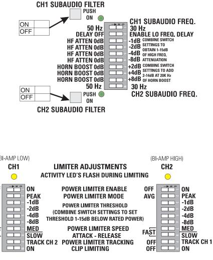
FOR STEREO TRACKING: ENABLE BOTH TRACKING SWITCHES.
