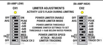
FOR STEREO TRACKING: ENABLE BOTH LIMITER TRACKING SWITCHES
