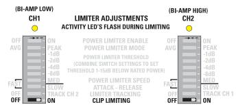
FOR STEREO TRACKING: ENABLE BOTH LIMITER TRACKING SWITCHES.
