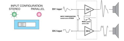
**PARALLEL:** The **CH 1** and **CH 2** inputs are connected together, applying a single input signal to both channels of the amplifier. A signal into any input jack will drive both channels. Each channel's subaudio filtering, clip limiting, and gain control still function independently. Each channel feeds its own speaker load.
