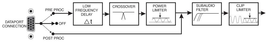
DATAPORT signal routing options using the DATAPORT INPUT SIGNAL switch
