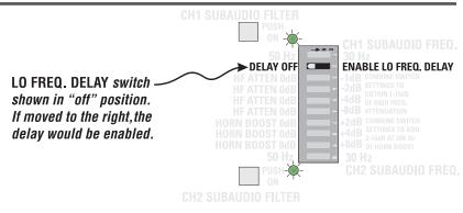
**HF ATTEN-** These switches are active only when the amplifier is in **BI-AMP** mode. These four switches (section 3, 4, 5, and 6 of the left-most DIP switch) work in combination to control the amount of high-frequency attenuation. The amount of attenuation can be selected in 1dB steps from 0 to 15 dB. Add the selected switch values for the total attenuation. EXAMPLE: Setting -1 dB and -4 dB results in -5 dB of high frequency attenuation.
