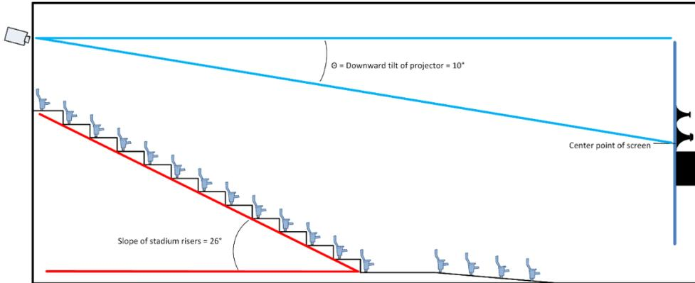
Figure 3 - Increasing stadium floor slope means raising the projector height, which in turn increases projection down angle – potentially increasing image distortion. Actual image distortion depends on multiple interacting factors, including image height, projection distance, screen angle (if any), lens type, etc.
