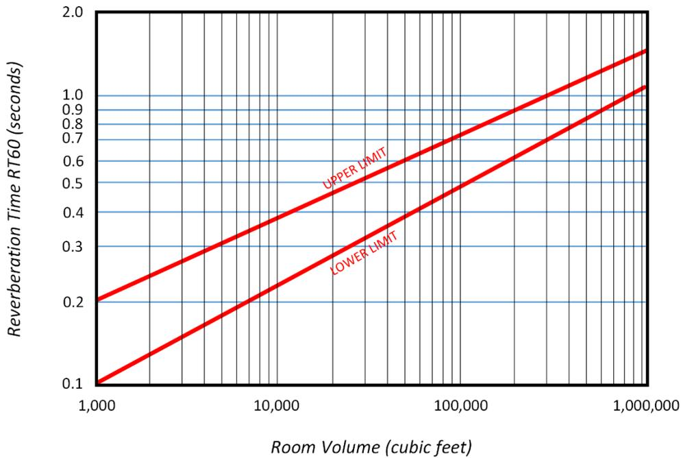
Figure 5 - This chart shows preferred reverberation times for the 500 Hz octave band for various room volumes.
