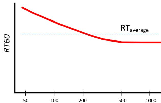
Figure 6 - Reverberation times are higher for low frequencies. It is typical for the reverberation time for low frequencies to be some 30% higher than the overall average broad-band reverberation time.
