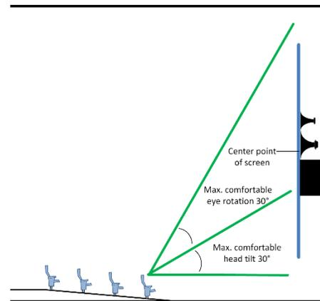
Figure 4 - Front row seated viewers (worst case) should not have to tilt their head more than 30 degrees, and should not have to rotate eyes upward more than 30 degrees.
