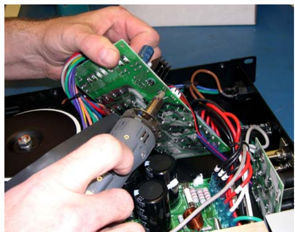
Figure 2. Unsoldering the wires.
