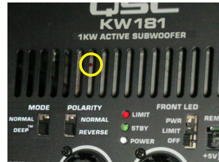
Figure 4. To show that the module has been updated, place a mark on the inside of the bucket where it will be visible through the slots.
