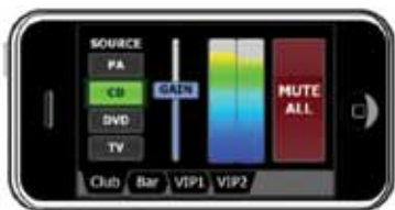
Custom control panel served on an iPhone.
