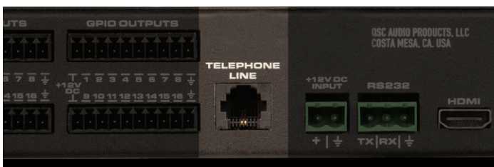
Figure 3. The POTS connection on the rear panel of the Core 110f.
